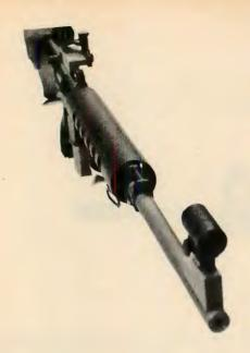
Note front sight blocks and no-contact, freefloating barrel.
